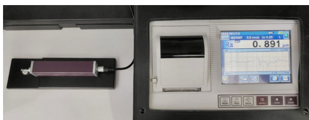
Fig. 2 Surface roughness assessment using surface profilometer (Mitutoyo SJ-310, Tokyo, Japan).
