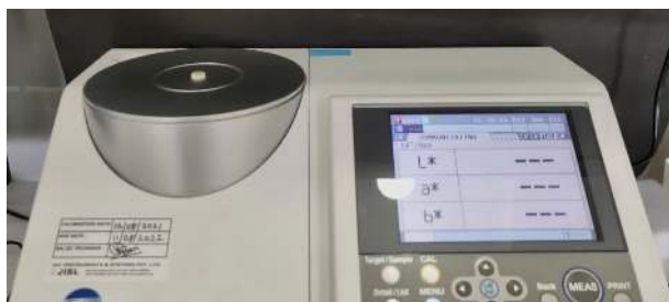
Fig. 1 Colorimetric assessment using Spectrophotometer (Spectrophotometer CM5, Konica Minolta, Tokyo, Japan).
