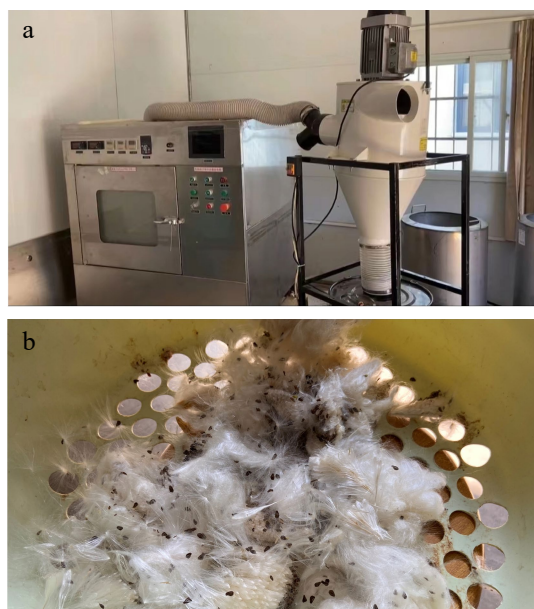
Fig. 2 (a) The CGF microwave-opening equipment. (b) The CGF extracted from microwave-opening.
