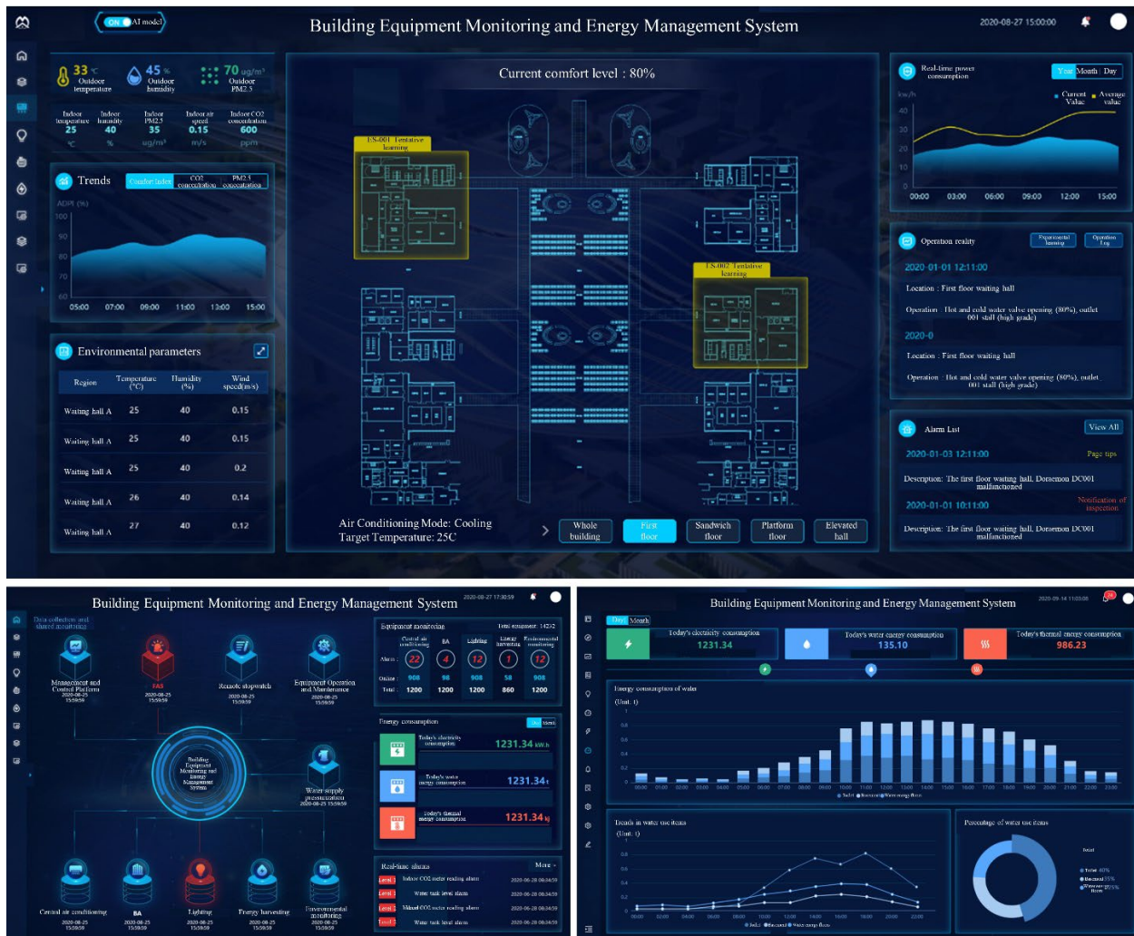
Fig. 6 Interface of building equipment monitoring and energy management system of the case station.
