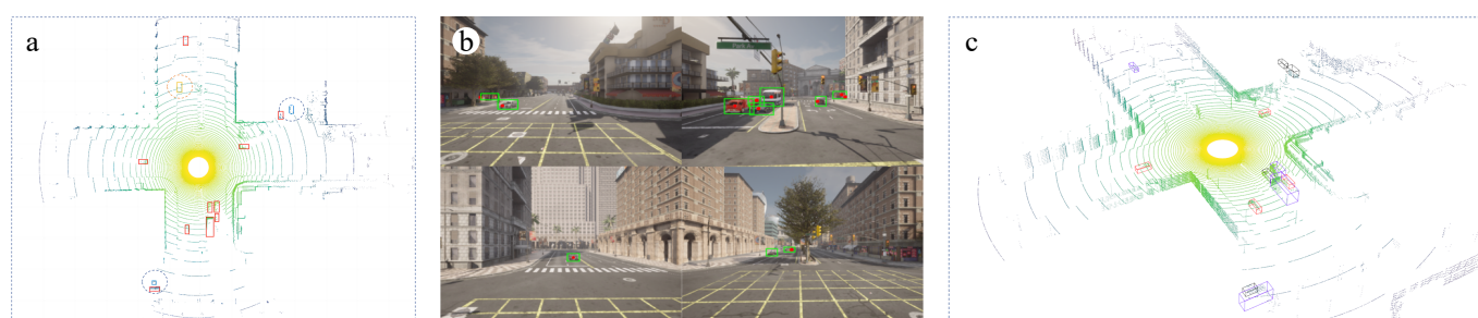
Fig. 5 Digital twin view. (a) BEV fusion view. (b) Camera view. (c) LiDAR view.
