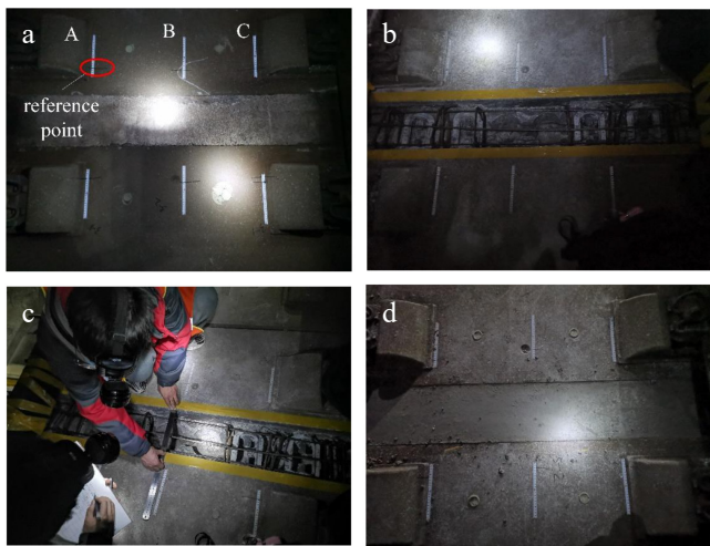
Fig. 13 Relative displacement measurement process. (a) Attaching a scale; (b) measuring distance; (c) measuring distance again; (d) measuring finished.
