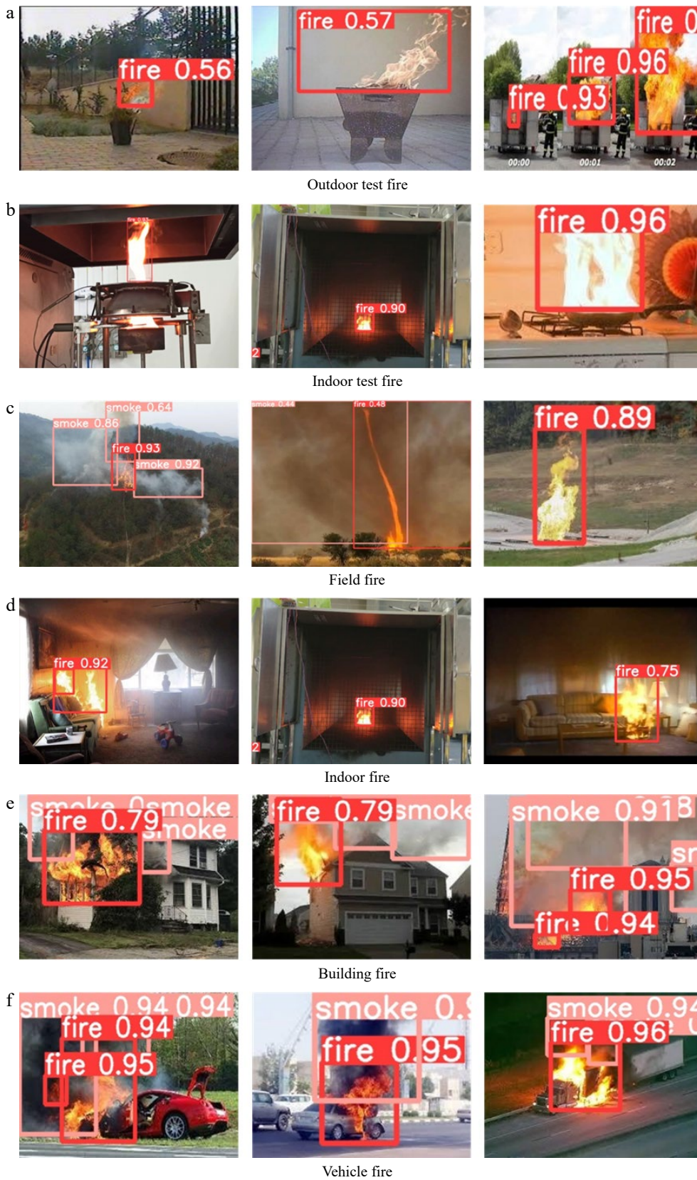
Fig. 12 Fire detection effects of the YOLOv5 + TR + \alpha CIU algorithm for different types of scenarios.
