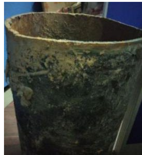
Fig. 1 Pipeline corrosion sample.
