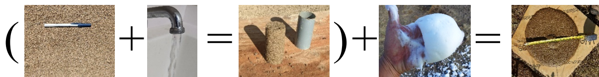
Fig. 10 Starting with pit run sand, water is added to raise the moisture content to 1%–2% below field moisture content, then preformed foam is added to about 30% vol/vol solids to produce a highly flowable, pumpable slurry mixture.
