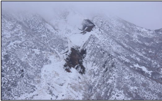
Fig. 4 South Canyon West coal mine fire, Colorado (USA) during snow. The coal bearing strata and mine workings plunge to the left at about 50 degrees and would be impossible to isolate.
