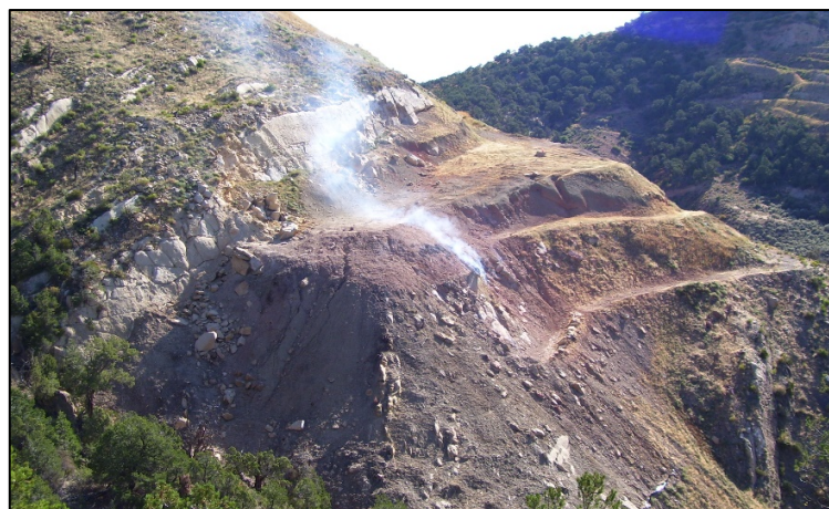
Fig. 9 IHI No.3 coal mine fire, Colorado (USA) which continues to burn vigorously despite multiple extinguishment efforts that included surface sealing, grouting and excavation.
