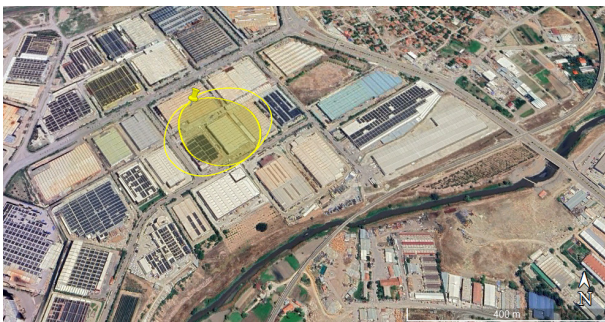
Fig. 4 Google Earth image of the explosion threat zone of the vapor cloud for hydrogen storage tanks (Scenario -1).
