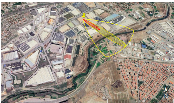
Fig. 6 Google Earth Image of the flammable threat zone of vapor clouds for hydrogen storage tanks (Scenario-1).
