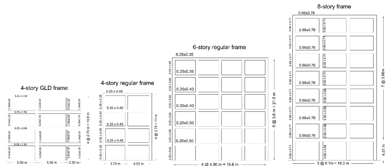
Fig. 1 Elevation view and cross section dimensions of the four frames under study.
