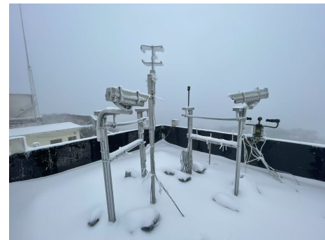
Fig. 3 The NH3000 automatic wire icing monitoring system and its installation setup.
