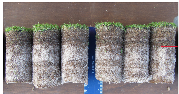
Fig. 1 Soil cores from an annual bluegrass putting green were evaluated from the zone below the green leaf canopy to the distinct interface between the thatch and sand layer indicated by the red arrow.
