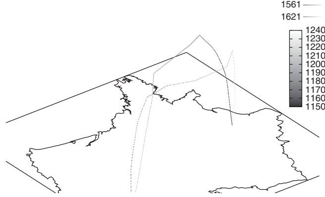
Figure 4 Three potential conflicts between two flights: one near Paris airport at low altitude and two other en-route at the cruising altitude of the lower flight. The grey scale corresponds to time (in minutes) along the trajectory, the lighter the later.
