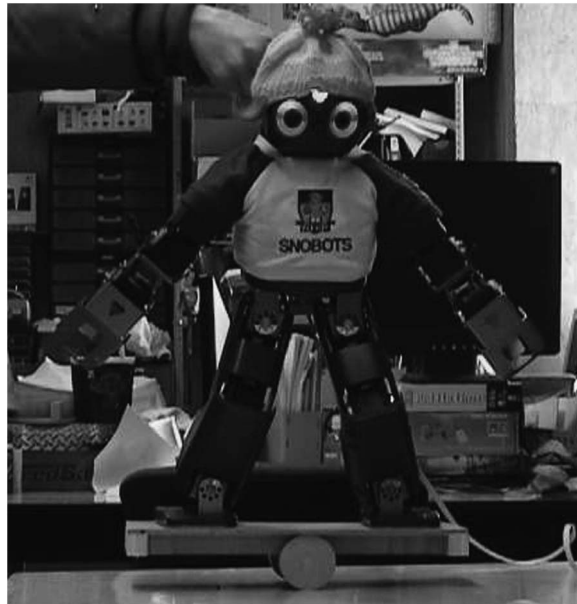
Figure 3 Jimmy, a DARwIn-OP humanoid robot, on a bongo board (Baltes et al. , 2014)
