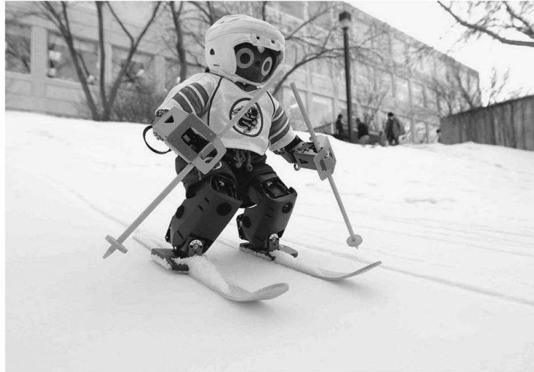
Figure 4 Jennifer, the robot used in this research, equipped with wooden skis and ski poles. The insulated shirt, helmet, and trousers helped protect the robot from cold and moisture (Martin, 2015)
