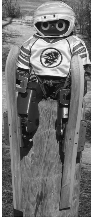
Figure 5 A detailed view of the skis used in this research. The skis are made out of spruce wood cut ~4 mm thick with steam-bent tips. The skis are attached to the underside of the robot's foot with counter-sunk screws to provide a smooth running surface
