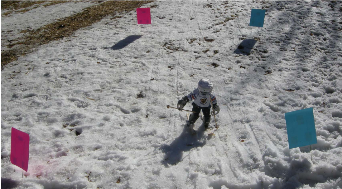
Figure 10 Jennifer navigating a simple skiing course. The robot is programmed to ski within the area marked by the markers to avoid going out of bounds
