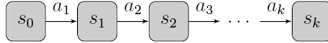
Figure 3 A solution to a planning problem as a sequence of actions and state transitions
