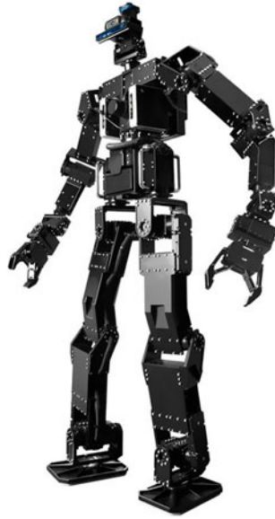
Figure 3 THORMANG3: Tactical Hazardous Operations Robot 3
