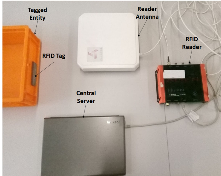
Figure 1 A typical RFID system consists of an RFID reader, which is connected to a reader antenna, an RFID tag and a central server.
