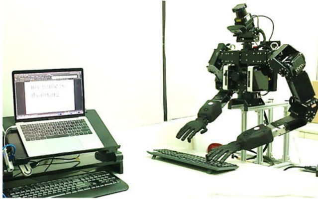
Figure 1. Modified THORMANG3 dual-arm humanoid robot to type with the keyboard
