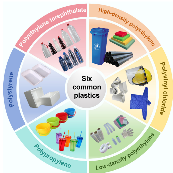
Fig. 1 Basic structure and product diagram of six common polymers (HDPE, LDPE, PP, PS, PVC, and PET).
