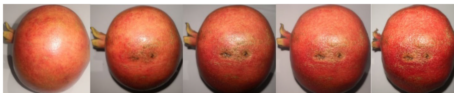
Fig. 1 Evolution of bruising damage over 8 d in pomegranate fruit (cv. Wonderful) that was dropped from 60 cm vertically (impact energy of about 1.8 J).
