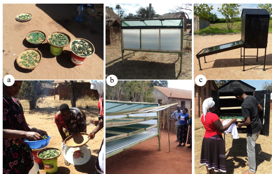
Fig. 2 (a) Open sun drying (traditional drying), (b) direct solar drying, and (c) indirect solar drying.
