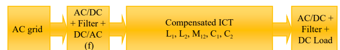
Fig. 2 Example of a static WPT for charging a battery from an AC grid.
