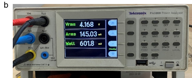
Fig. 7 Experimental waveforms under 600 kHz operation frequency and 27 Ω load resistance. (a) Experimental waveforms, (b) measured output voltage, current, and power.
