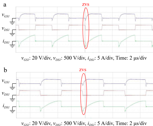
Fig. 24 Various waveforms of power switch Q_1 with output voltage of 280 V and 340 V in forward charging CC mode. (a) V_{DC\_Grid} = 400 V, V_{Bat} = 280 V, I_{Bat} = 2.5 A. (b) V_{DC\_Grid} = 400 V, V_{Bat} = 340 V, I_{Bat} = 2.5 A
