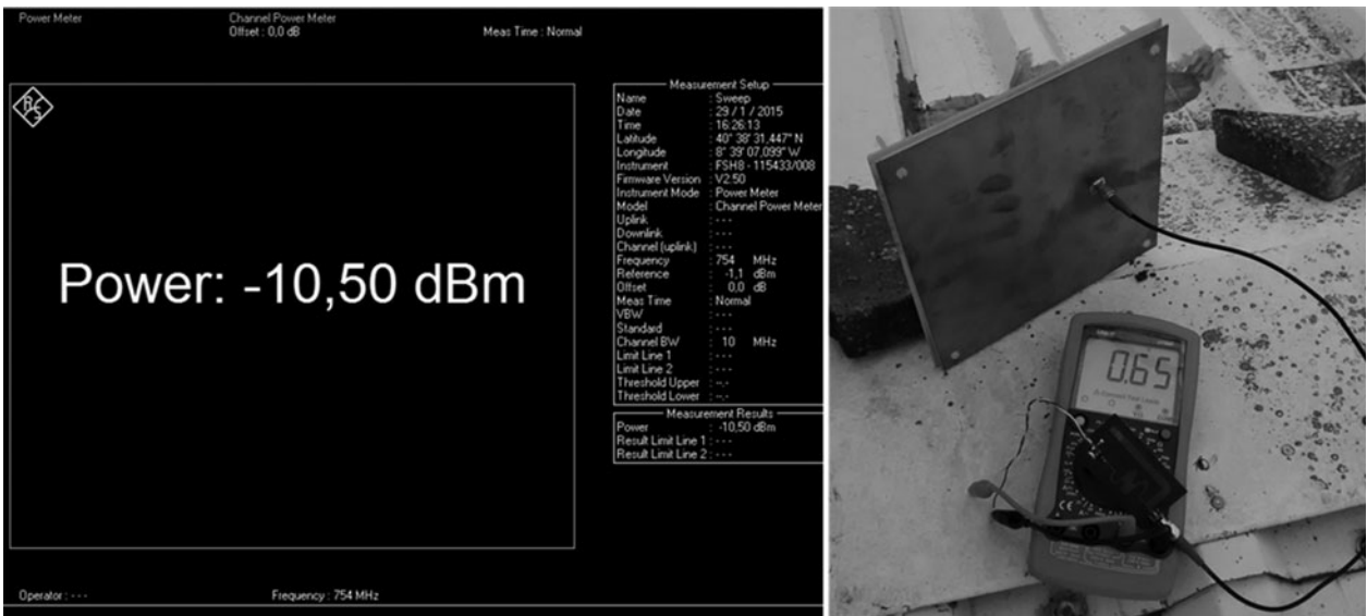
Fig. 15. Power received by the antenna (left) and output DC voltage at the voltage doubler (right).
