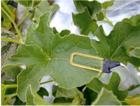
Fig. 5. Temperature sensor applied to a melon leaf.
