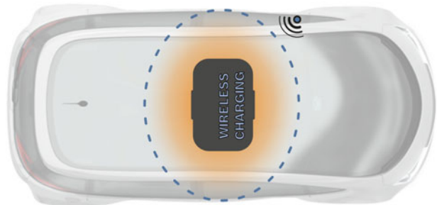
Fig. 3. Inductive charging pad containing the primary coil below an EV that is equipped with a sensor at its underbody to monitor the whole protection area (blue, dashed).
