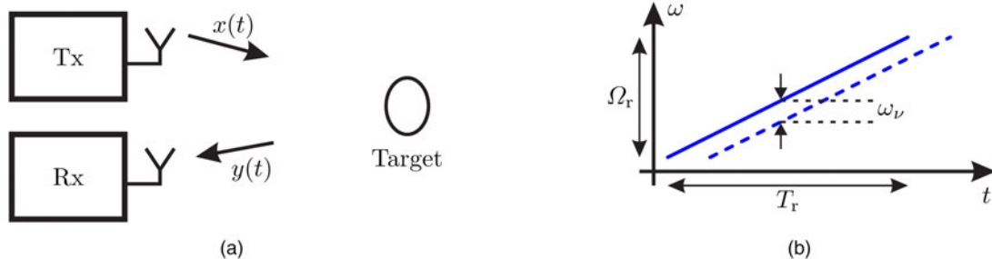
Fig. 5. Principle of FMCW radar sensors. (a) Block diagram of a principal radar system with transmit and receive signals x(t) and y(t) , respectively. (b) Frequency difference \omega_v resulting from x(t) (solid) and y(t) (dashed).
