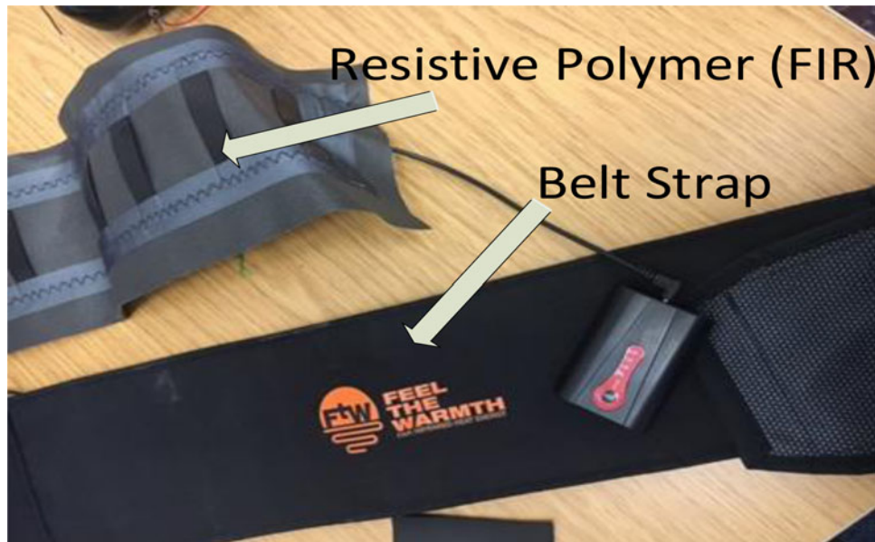
Fig. 2. Wearable belt with the charging element.
