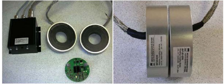
Fig. 15. INPUD DON100 HE30 underwater inductive charging equipment [30].
