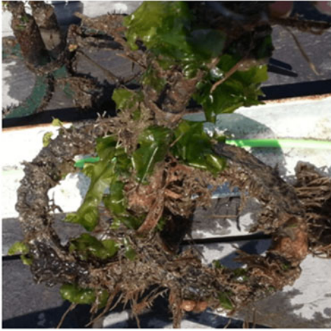
Fig. 11. Bottom of control coils (no Anti Foul) after 45 days [19].
