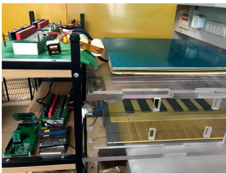
FIGURE 9: Experimental setup for wireless power transfer under inhomogeneous winding.
